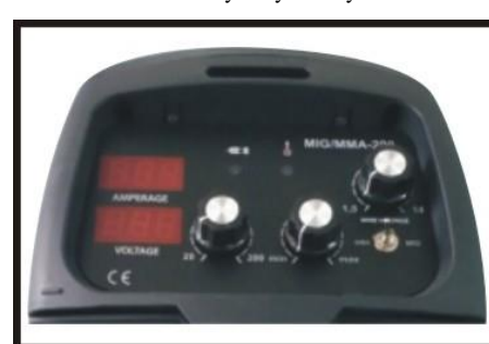
(20) Set welding parameters using the voltage and wire feed controls.
