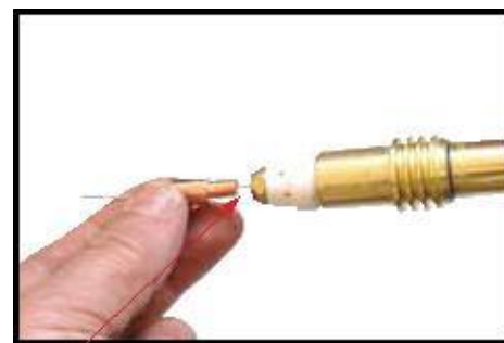
(17) Fit the contact tip over the wire and screw it into the tip holder, nip it up tight.
