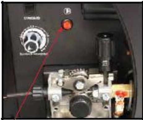
(12) Press and hold the inch wire button to feed the wire down the torch cable through to the torch head.
