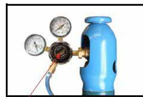
(19) Carefully open the valve of the gas cylinder, set the flow to 15 - 25 CFH
