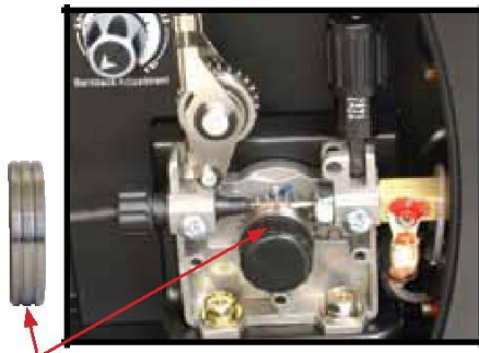
(11) Install a U groove drive roller of the correct size for the diameter wire being used.
