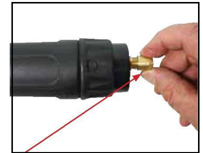
(6) Fit the liner retaining nut and screw only 1/2 way down
