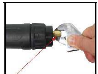
(9) Fully screw down the liner retaining nut and nip it up tight.
