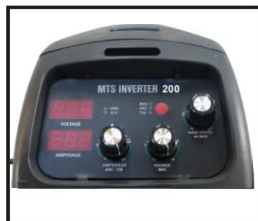
(16) Set welding parameters using the voltage and wire feed controls.
