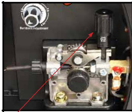
(10) Apply a medium amount of pressure to the drive roller
